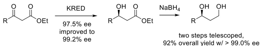
In this reaction, the step1 is a KRED catalyzed enantio-selective reduction of ketone, and the step2 uses NaBH<sub>4</sub> to furnish a second hydroxyl group. The initial hit in PharmaBlock's in-house enzyme stock gave 97.5% ee, with roughly 1% ketone remaining after 5 hours reaction. This screening outcome is very promising though the
