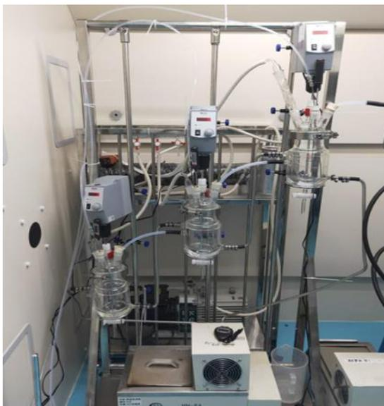
Figure 7 A three-stage MSMPR crystallizer.
