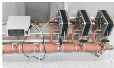
Plate Carbide Tubular Reactor
