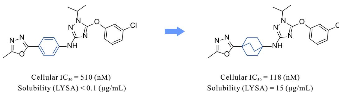
**Figure 4.** Effect on Potency and Developability Parameters of Bioisosteric Replacement of a phenyl ring of  $\gamma$ -Secretase Modulator with a BCO Moiety
