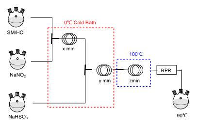
Figure 6. Scheme of Hydrazine preparation via diazotization
